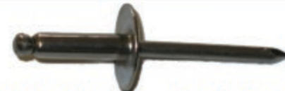
3/16 X .575 .251-.375 GRIP SS RIVET LARGE FLANGE
