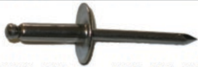
3/16 X .700 .376-.500 GRIP SS RIVET LARGE FLANGE
